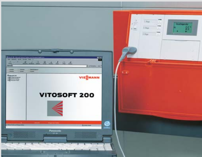
Vitsoft 200 ServiceControl and Optolink interface – for easy commissioning, maintenance and service
